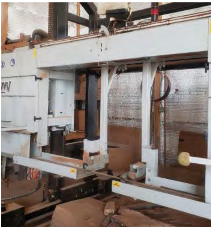
67" diameter Wood-Mizer Saw, WM-1000. One of the largest saws of its type in the Mid-Atlantic.
